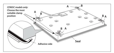
Note: if your bench is thicker than 40 mm, recess the underside to between 30 and 40 mm.
